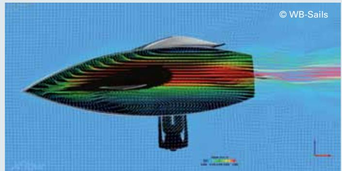
Figure 2: Flow in a plane 10 cm below the surface. The red arrows all point forward, even if you may not see it at the print resolution. If you look close, you can see the quarter wave on the leeward side, where the arrows change direction abruptly.
