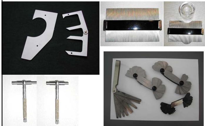
Special tools: sheerline, radius, inside dimensions.
