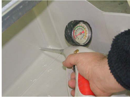
Buoyancy tank air test
