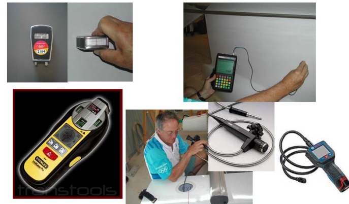
Very Special tools: Metal detector, optical fiberscope, magnetic and ultrasonic thickness gauges.
